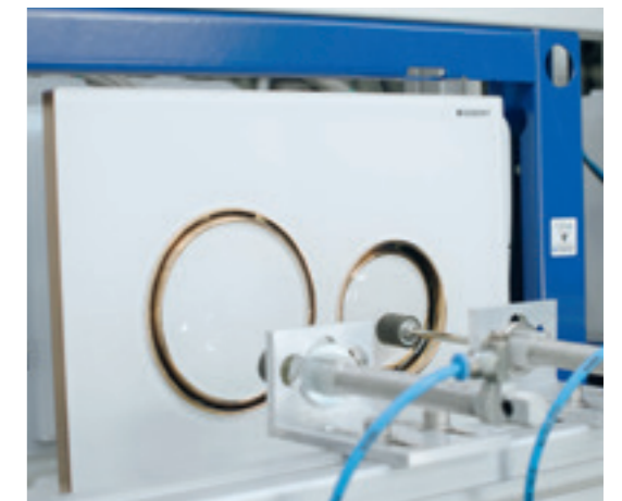
↑ LOAD TESTS Geberit ceramic must pass stringent load tests and reliably fulfill all relevant standards.
