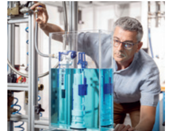
↑ HYDRAULICS EXPERTISE Geberit's sanitary technology laboratories put flush and fill valves through their paces to demonstrate maximum hydraulic performance and pass long-term durability tests.
