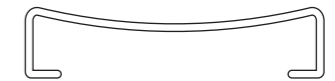
↑ The concave profile curves inward, helping transport water quickly and efficiently to the central drain without a slope.
